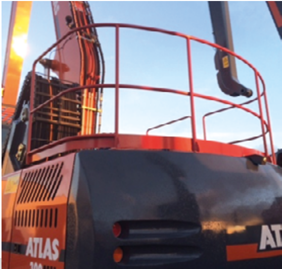
HANDRAIL FOR SUPERSTRUCTURE
