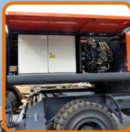
Control cabinet for E-Drive
