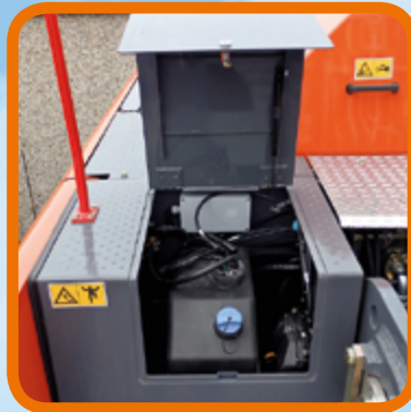
Easily accessible AdBlue® tank
